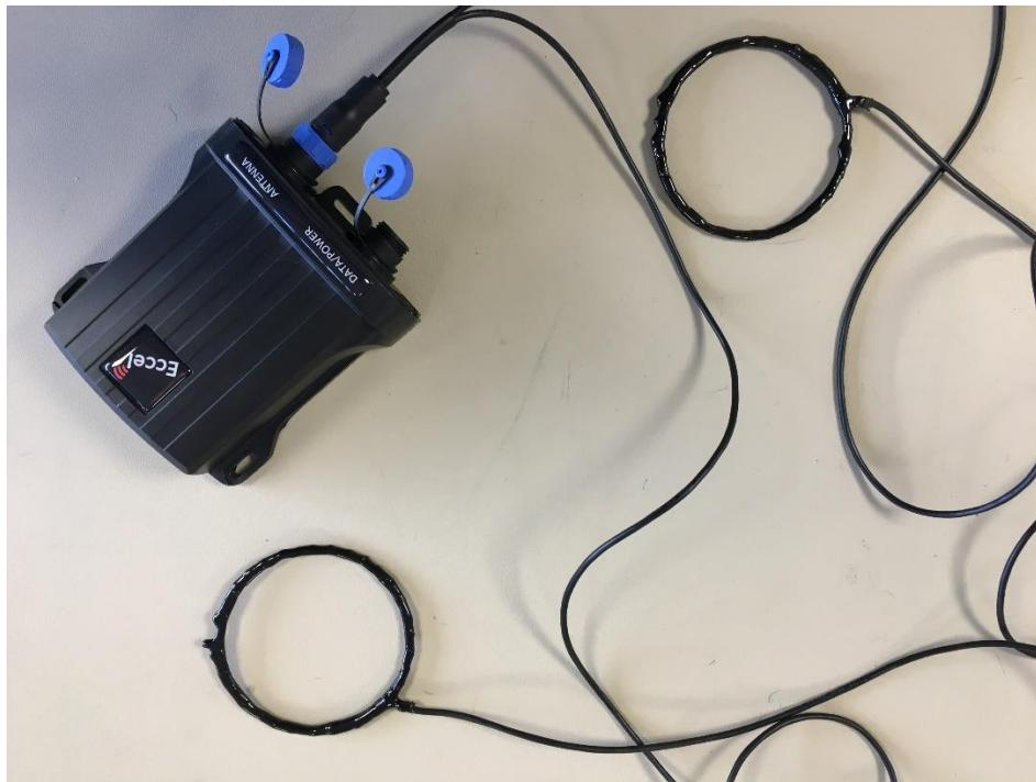
3. Connect the lead for the datalogger/battery unit to the RFID unit:
