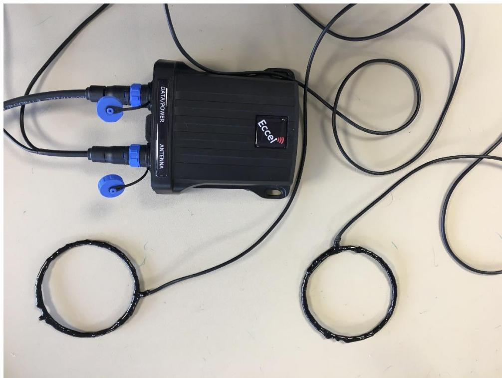
4. Now connect the other end of the data/power cable to the datalogger/battery unit. Once this connection is made, the system will be running and looking for tags (currently at the
