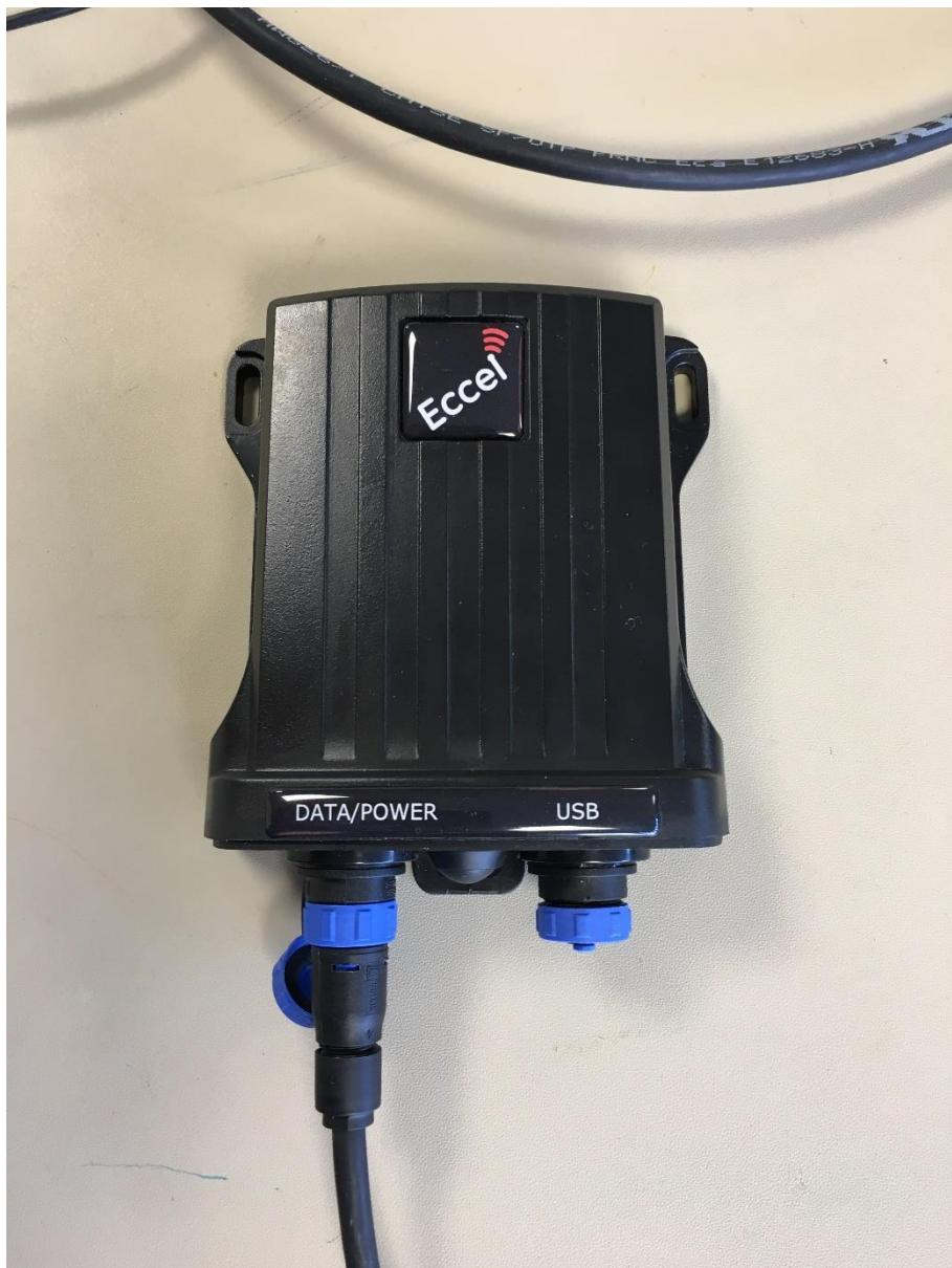
5. The range test can now be performed by connecting over Wi-Fi to the RFID unit from a PC or tablet by firstly powering up the Wi-Fi of both the RFID unit and the datalogger/battery unit by pressing and holding the button on the datalogger/battery unit for at least 3 seconds. The red LED in the button will illuminate when the Wi-Fi is enabled.
