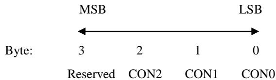
The Hitag S configuration bytes indicate the type of HS transponder and the mode of operation. Please note that the MicroRWD H1/S module only supports Plain Memory mode (default mode as set by Philips). Configuration bytes also control whether the memory blocks are read/write or locked for read only access.
