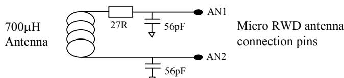
The 27 ohm in-line resistor reduces the peak antenna voltage to 200 volts peak-to-peak (125kHz antenna) to ensure optimum signal to noise ratios are maintained for best performance and range.
