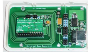
3) Select the appropriate 125 kHz antenna coil or on-board 13.56 MHz PCB antenna type by fitting links to 6-pin header according to the diagram below:
